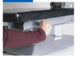
Insert Heated Lower Platen spindle and secure.
