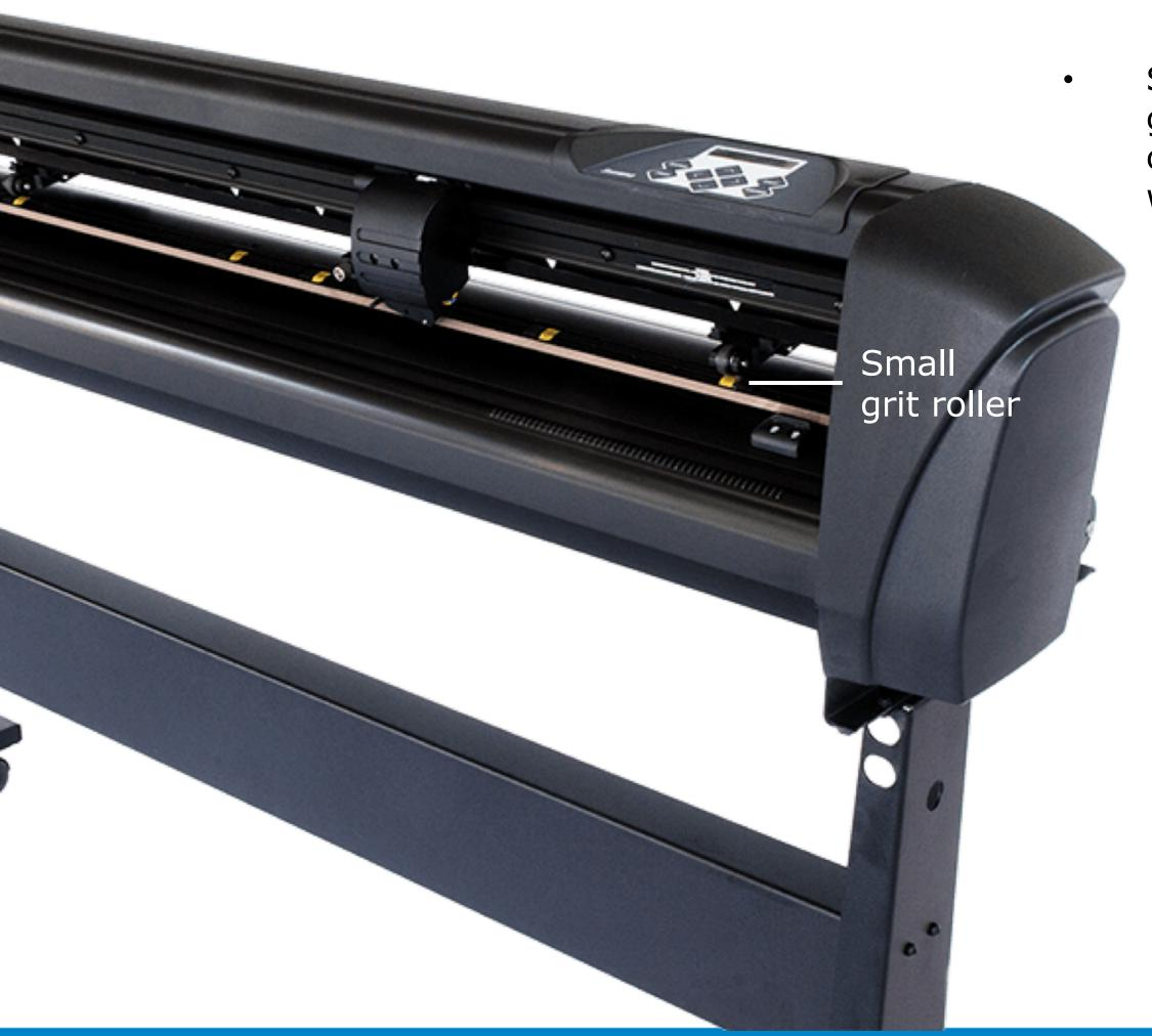
Similar to the SummaCut D60FX, the SummaCut D140RLFX has no wide grit roller. The SummaCut D140RLFX has 6 small grit rollers that are optimally placed so that most common media formats can be handled with ease.
